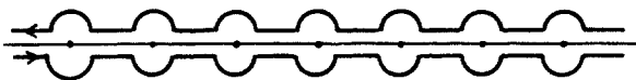
Figure 1. Path taken for the integral appearing in equation (8). The dots correspond to the poles of G(\omega_0) .
